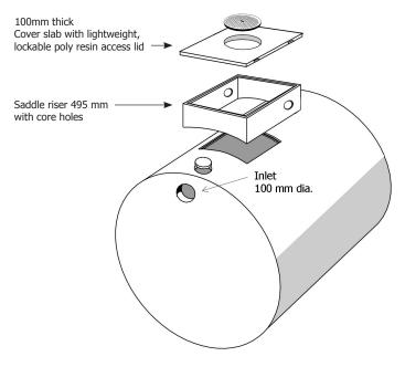
The tanks have been designed to be buried with the top of the tank located 900mm maximum below ground level and with the cover slab at ground level.
